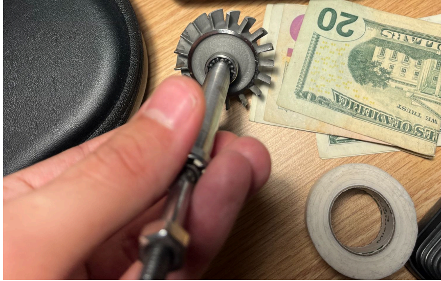
Turbine assembled onto shaft with bearings for balancing
